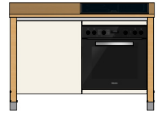
Herdumbau/ Türli. bloc 430THR/Br. 103cm/li 30 bloc 531THR/Br. 118cm/ li 45 bloc 530THR/Br. 133cm/li 60
