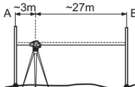
**Step 3:** Aim at Staff B and press MEAS key. Measurement display, press and hold measuring key for 3 seconds to accept.
