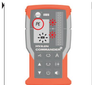
LEDs and the AUTOALIGN symbol start to flash while COMMANDER 2 HVA2N searches the laser beam. The LCD shows an >> PE <<.
