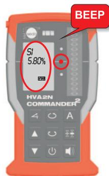
After AUTOALIGN single has finished, grading of the Y-axis is shown in the LCD (e.g.: 5,80%)
